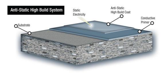
Anti-Static High Build System is a high build static dissipating colored epoxy coating system. It is used for environments where static control is needed.
