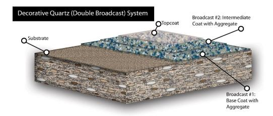
Decorative Quartz Double Broadcast System is a decorative, multi-lift, high strength concrete resurfacing system. It is used for environments requiring an attractive, high performance floor or when a concrete floor has sustained damage requiring a textured 1/8" surface restoration.
