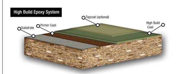
High Build Epoxy System is a high build, colored epoxy/urethane, high performance concrete coating system. It is used for environments requiring an attractive, high performance floor or when a concrete floor has sustained damage requiring a moderately thick resurfacer.
