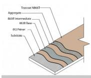
Primer/Sealer: NP013, Two Component, Water based Epoxy Primer/Sealer Base Membrane: NP863B, Non-Gassing, Single Component, Moisture Cured Polyurethane Membrane
