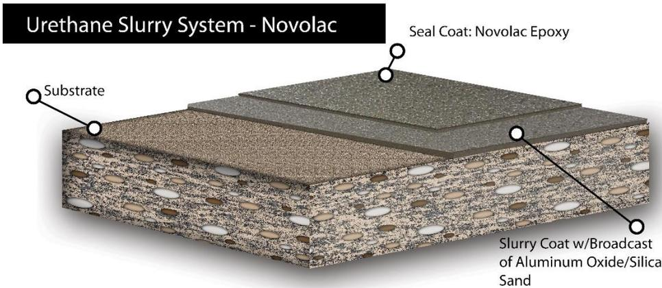
Urethane Slurry System is a self-leveling, low odor slurry that can be applied at 1/8" thickness and broadcast to yield a 3/16" system. It is used for environments requiring a durable floor that can withstand heavy and abusive service. Urethane slurry systems are an ideal choice for resurfacing areas where a durable shock resistant surface is needed.
