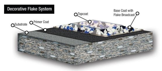
Decorative Flake System is a decorative and extremely durable concrete resurfacing system. It is used for environments requiring an attractive, aesthetically pleasing, high performance floor.
