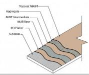
**Primer/Sealer:** NP013, Two Component, Water based Epoxy Primer/Sealer **Base Membrane:** NP863B, Non-Gassing, Single Component, Moisture Cured Polyurethane Membrane
