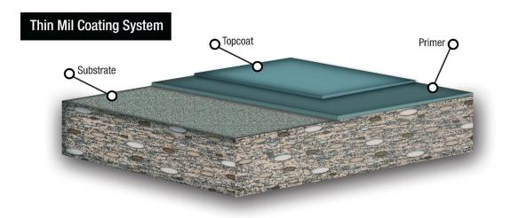
Thin Film Industrial Floor is a colored epoxy/ concrete coating system. It is used for environments requiring an attractive, economical, high performance floor. Satin finish
