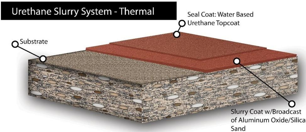
Urethane Slurry System is a self-leveling, low odor slurry that can be applied at 1/8" thickness and broadcast to yield a 3/16" system. It is used for environments requiring a durable floor that can withstand heavy and abusive service. Water Based Urethane Topcoat provides additional thermal shock capabilities.
